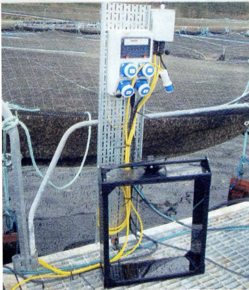
Top and right: Vaki's Biomest system takes a real-time picture of the size and distribution of fish in each cage
